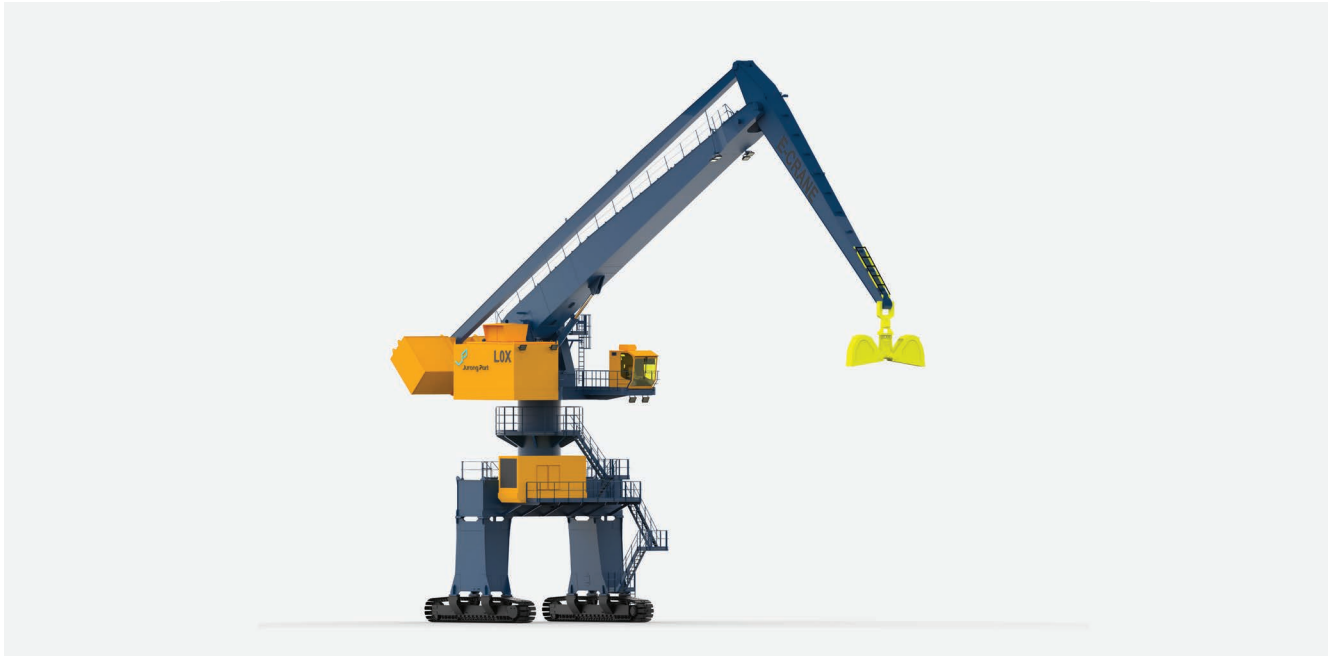
▲ An artist impression of electric balance cranes that will be used for aggregates handling at Jurong Port by 2022.
