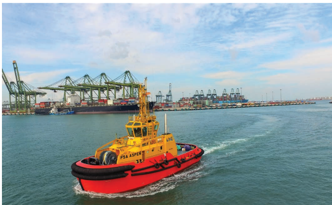
▲ PSA Aspen, PSA Marine's first dual fuel LNG harbour tug.
