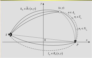
Denoted by an intermodal route. It may consist of a sequence of nodes (i.e., points) as well as the links between two consecutive nodes in the x-y plane. A node can either represent a transfer node where containers are switched between different modes or a location where the handling of containers does not happen. The latter is referred to as regular node. One example regular node is the interaction
